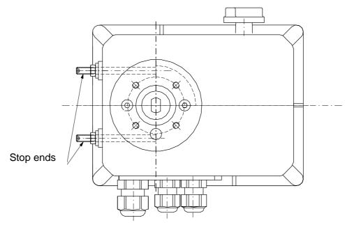
Fig.8: Flange of actuator from bottom.
